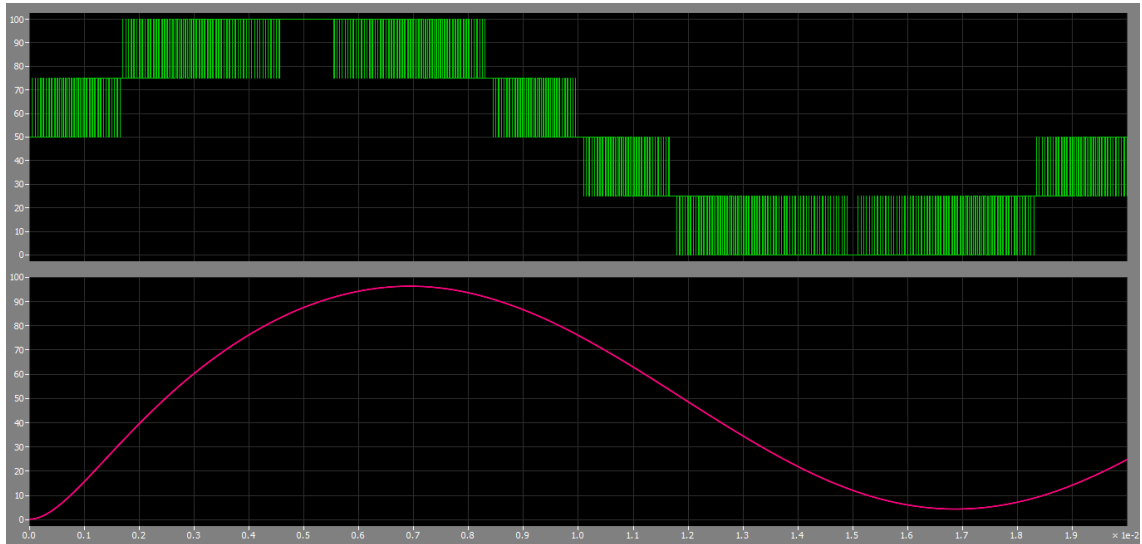
Figure 4.7: Simulation results given by the PLECS model: output voltage V_{out} (upper subplot) and filtered voltage across C_L (lower subplot).
