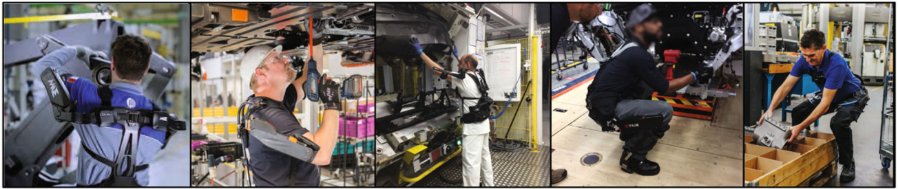
Fig. 1 Examples of assistive devices for manual tasks in the manufacturing industry. From the left: the Mate [19], the AirFrame [20], the ShoulderX [21], the LegX [22] and the Laevo V2 [23]
