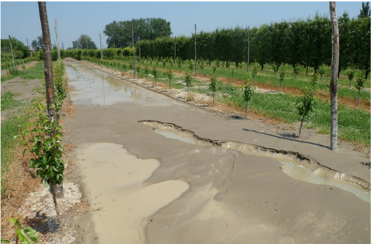
Fig.4. Example of liquefaction-induced ground surface effects observed in Cavezzo after the 29th May 2012 earthquake with 5.8 magnitude.
