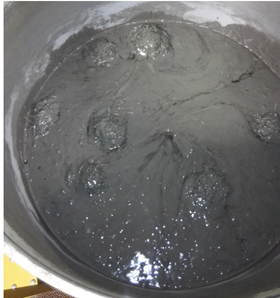
Figure 2.8: Phenomenon of fiber balling occurred in M1-HF65-5, M1-HF85-5 and M2-HF85 series
