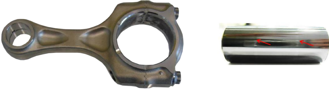
Figure 6.1. Conrod and piston pin of the engine under investigation.
