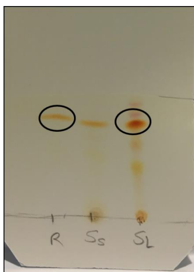
Figure 76. TLC of reduced VQ10. R_f, 3 = 0.55 , R_f, 2 (Disperse Orange 3) = 0.74 (hexanes - ethyl acetate 1:1 v/v)
