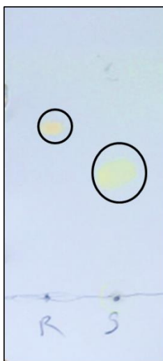
Figure 72. TLC of reduced DO3. R_f,3 = 0.55, R_f,2 (Disperse Orange 3) = 0.74 (hexanes - ethyl acetate 1:1 v/v)
