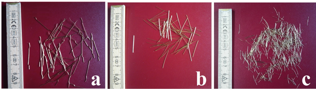
Figure 1: Steel fibers used in the mortars: a) Hooked fibers 30/0.35 mm; b) Straight fibers 20/0.3 mm; c) Straight fibers 13/0.175 mm.
