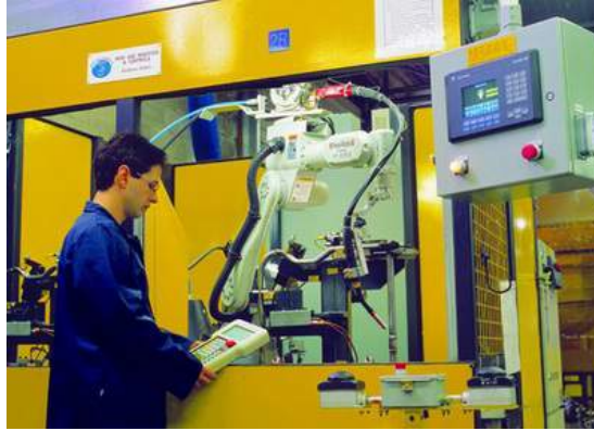
Figure 9: Lead-through programming by teach pendant.
