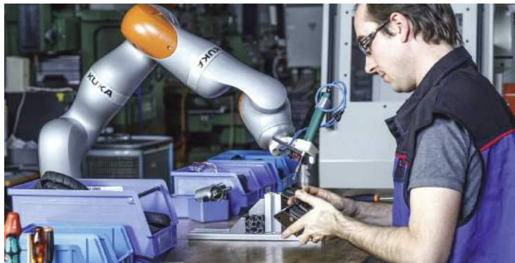
(b) Collaborative robot allowing the human worker to stand in its proximity and work together at the same task.
