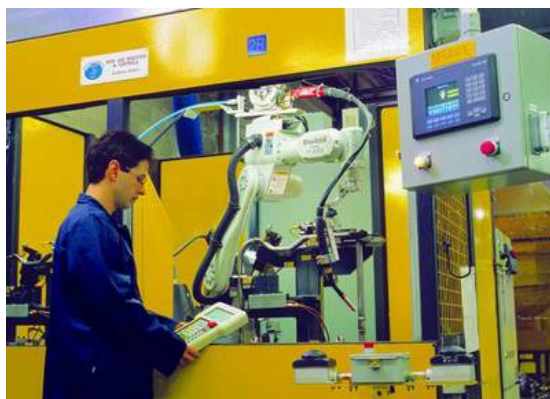
Figure 9: Lead-through programming by teach pendant.
