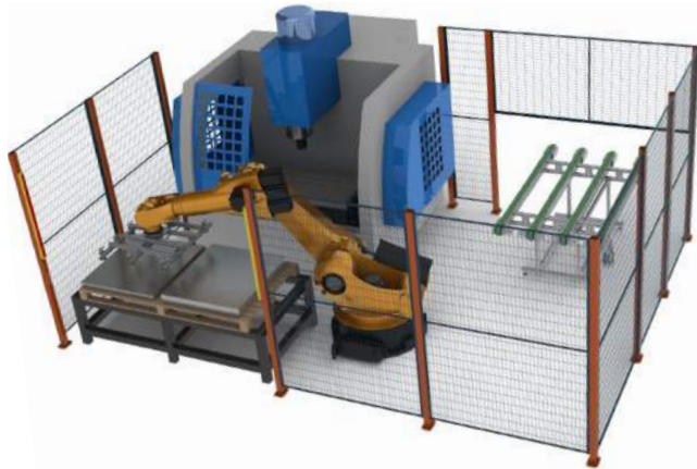
(a) Non-collaborative robot: safety fences are required to prevent harming human operators.
