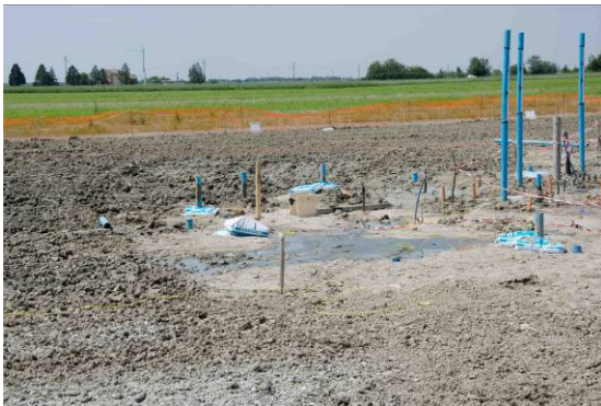
884 Figure 7. Blast-induced sand boils after the 885 first detonation.
