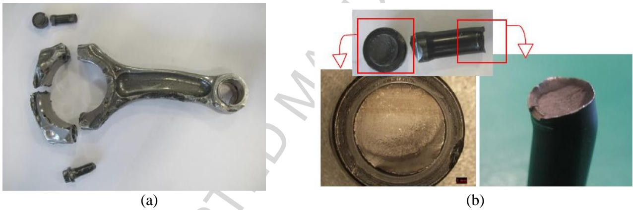
Fig. 18. Fatigue crack in the bolt:(a) global view; (b) bolt detail.
