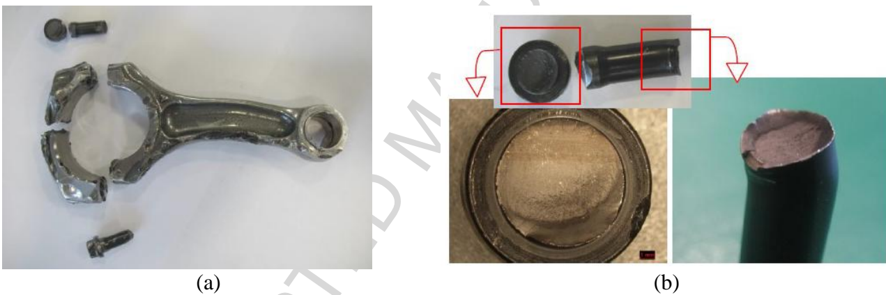
Fig. 17. Failure of the bolt connection: fatigue crack in the cap: (a) global; (b) detail; (c) undesired stress concentrations in the big-end induced by through screws: maximum principal stress distribution.
