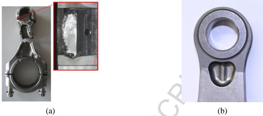
Fig. 13. Fretting in con-rod small end: (a) fatigue crack in con-rod small end; (b) titanium con-rod small end with DLC anti-fretting coating.
