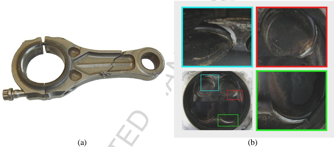
Fig. 4. Unusual 45° fatigue crack in the con-rod shank (a); contact between the piston and the valves due to torsional deflection of the con-rod (b).
