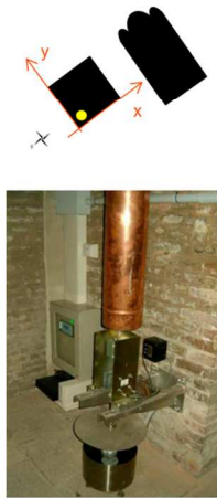
The observation reference system, picture and location of the dual-axis pendulum which is installed inside the Tower since 2003 (left); the pendulum time series representing the overhang trend in the same time span investigated by the proposed methodology (right). 118x56mm (300 x 300 DPI)
