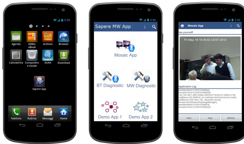
Fig. 7. Screenshots from the Android SAPERE App. (left) The launch icon to be pushed on the Android springboard to start SAPERE and have that device to become a node of the ecosystem. (center) The user is presented a menu of the locally available SAPERE services; launching one of them brings to life the associated agents and their LSAs. (right) the GUI of a simple test application for inspecting the LSA space.
