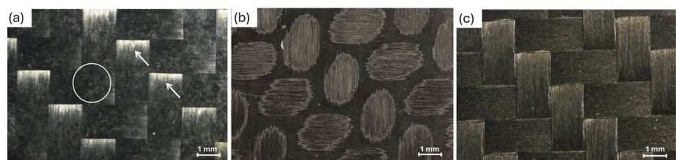
Fig. 3 Stereoscopic images of CFRP surfaces: (a) untreated, (b) laser cleaned, and (c) laser ablated
