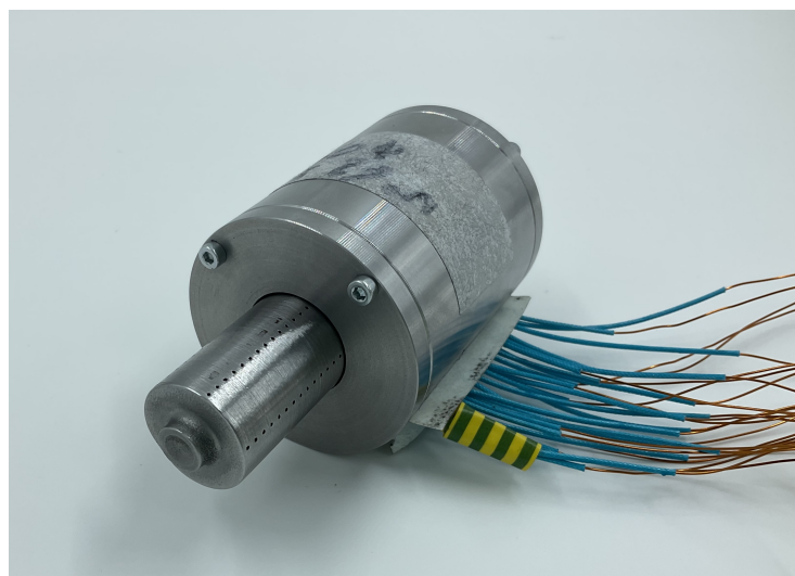
Figure 19. Fabricated linear motor prototype.
