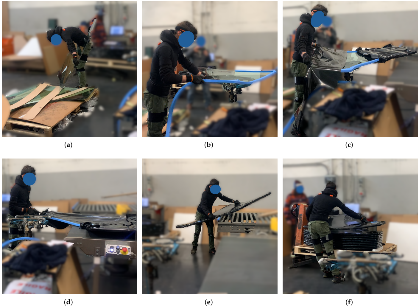
Figure 4. Windshield refinement workstation tasks. (a) The operator lifts up the windshield from the pallet. (b) The operator applies a protective foam border. (c) The operator wraps the windshield. (d) The operator puts the windshield onto the conveyor. (e) The operator lifts up the windshield from the conveyor. (f) The operator puts the windshield on a pallet.
