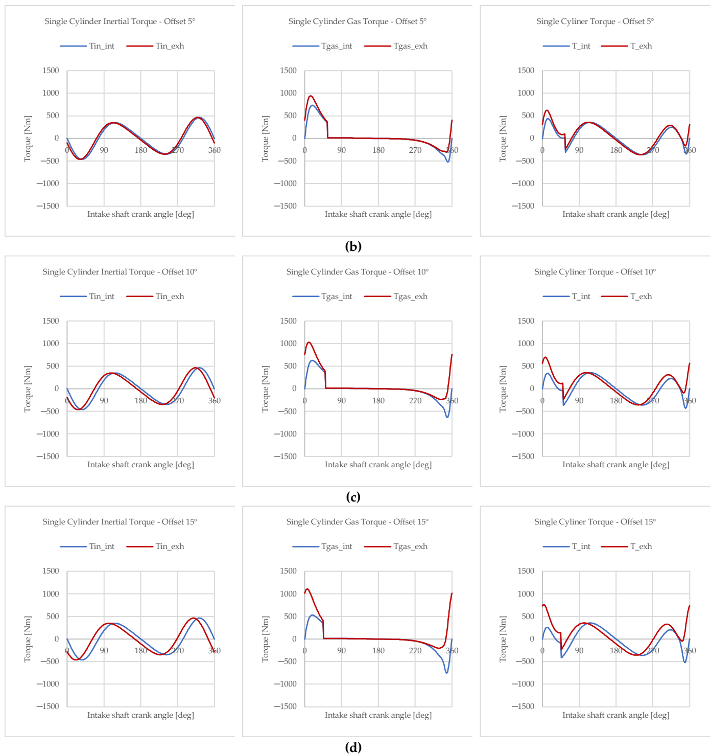
Figure 13. Output torque of a single cylinder; (a) 0° offset; (b) 5° offset; (c) 10° offset; (d) 15° offset.
