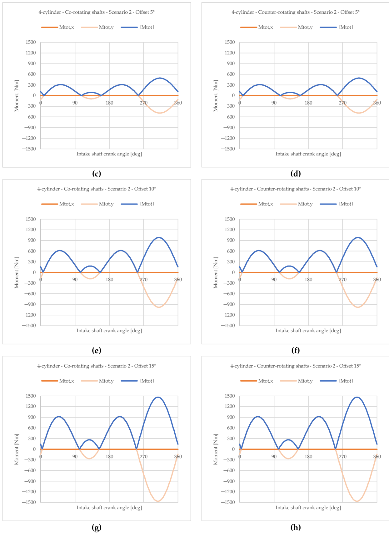
Figure 10. Resultant moment of co-rotating and counter-rotating shafts with M'_{rec,r} unbalanced (scenario 2) and with different offset angles for 4-cylinder configuration; (a) co-rotating with 0° offset; (b) counter-rotating with 0° offset; (c) co-rotating with 5° offset; (d) counter-rotating with 5° offset; (e) co-rotating with 10° offset; (f) counter-rotating with 10° offset; (g) co-rotating with 15° offset; (h) counter-rotating with 15° offset.
