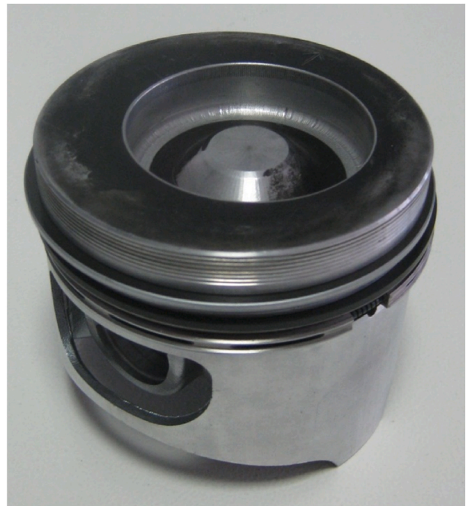
Fig. 1. Piston with modified bowl [26].
