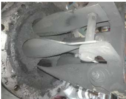
Figure 9a. Soot deposition on the top of the HX: rack of twisted tapes after the tests.
