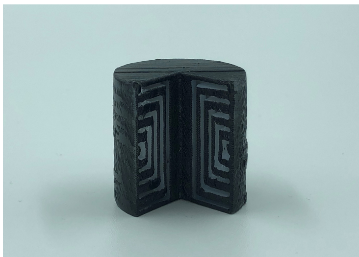
Figure 2. Additively manufactured mock-up prototype of the plunger pole of the synchronous tubular machine with five layers [22].
