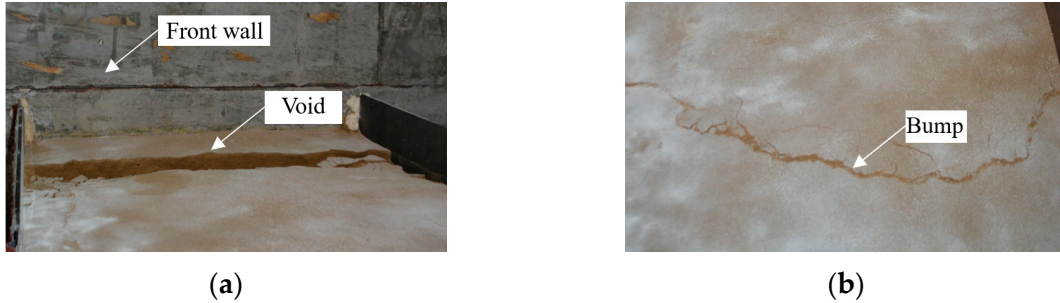
Figure 8. Sand surface deformation in H63-Push: (a) void near the proximal end; (b) bump near the distal end.
