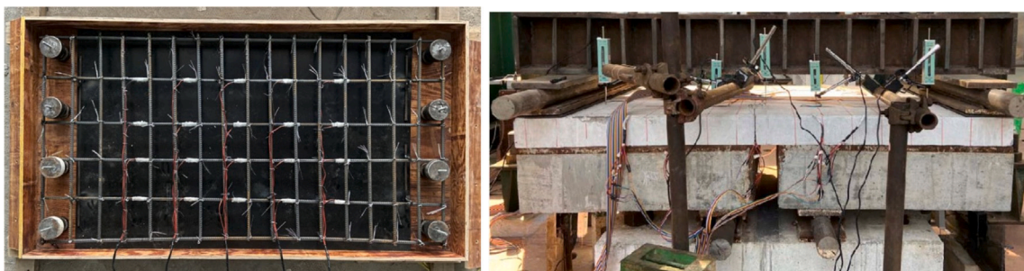
Fig. 9. (a) Installation of the strain gauges on the steel rebars, (b) experimental setup with all installed transducers.
