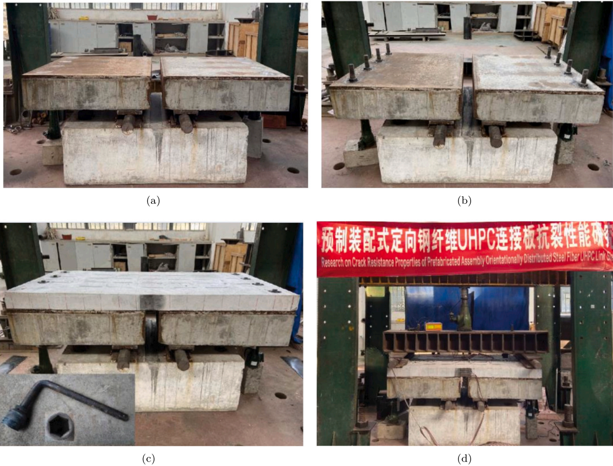
Fig. 7. Selected phases of the assemblage process: (a) shows the two girder segments with L-shaped steel profiles, (b) the welding of the bolts, (c) the fastening of the link slab and (d) the positioning of a steel beam for the four-point bending tests.
