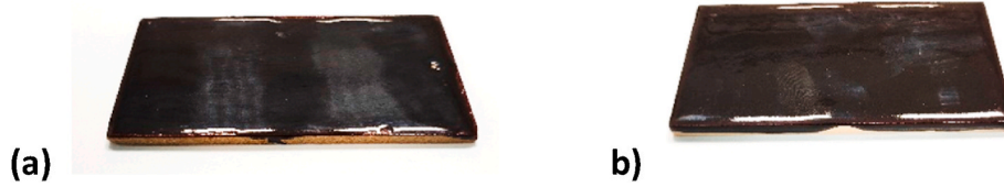
Fig. 5. Tile glazed with glaze formulation 7 (a) and 8 (b) after firing.
