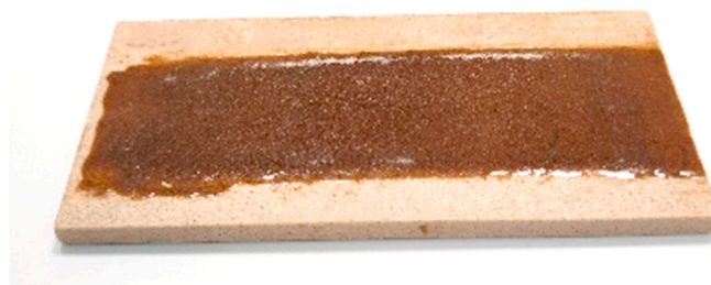
Fig. 3. Tile glazed with glaze formulation 3 after firing.
