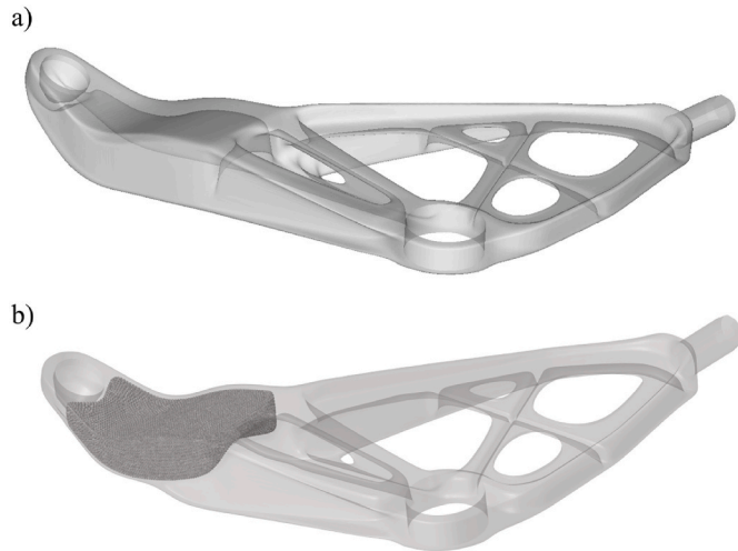
Fig. 3. Case study in the bulk (a) and lattice (b) versions. Box dimensions 253 × 154 × 329 mm.
