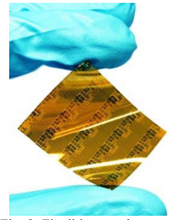
Fig. 2. Flexible complementary circuits and thin-film transistors on a 50 µm thick polyimide foil.
