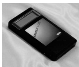
Figure 1. EMDEX Lite personal dosimeter (Enertech Consultants, Campbell, CA, USA) used to assess and monitor exposure to power frequency (50/60 Hz and their harmonics) magnetic fields in groups of workers
