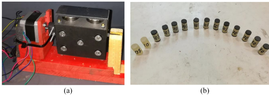
Figure 3. (a) Rotation system to prevent settlement of the particles, and (b) specimens manufactured.
