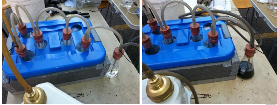
Figure 3. Tar and particulate sampling apparatus before (left) and after (right) the test.
