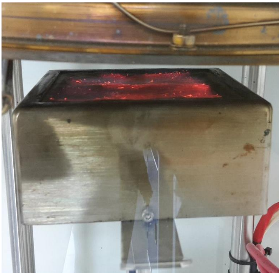
Fig. 11: FRAB-based insulation material during cone calorimetry testing.
