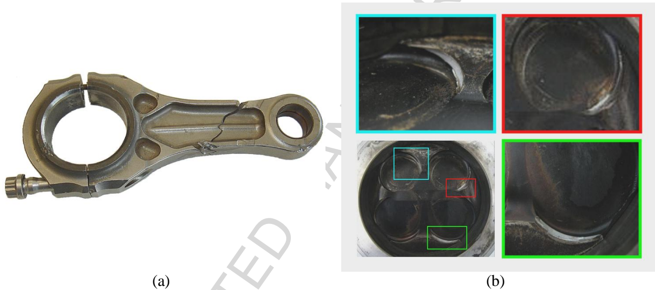
Fig. 4. Unusual 45^\circ fatigue crack in the con-rod shank (a); contact between the piston and the valves due to torsional deflection of the con-rod (b).
