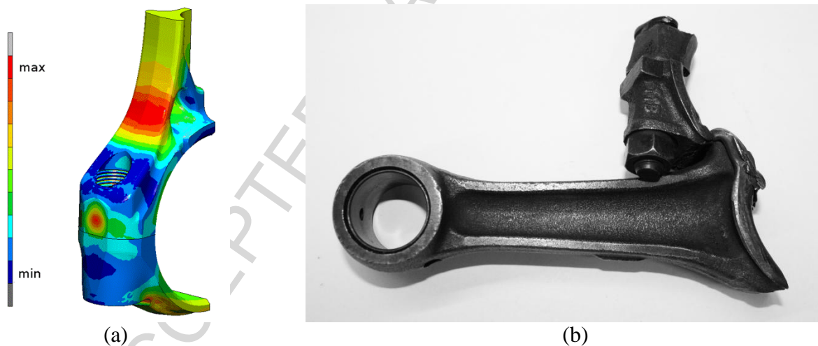
Fig. 16. FE analysis of the stress field within a con-rod big end: distribution of the maximum principal value of stress (a); fracture in con-rod big end (b).
