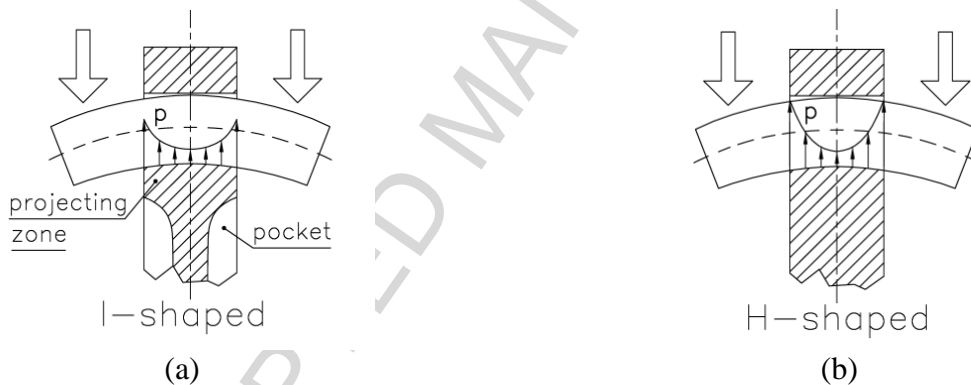
Fig. 6. Influence of the shank geometries on pressure peaks at the contact between gudgeon pin and small end bore: (a) I -shaped shank; (b) H -shaped shank.
