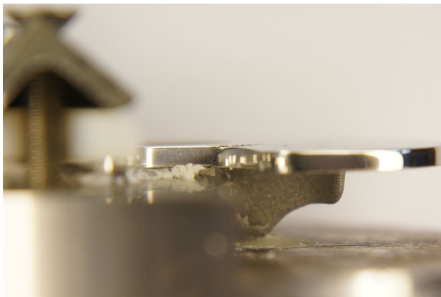
Fig. 9 Fatigue crack observed in the frontal plane
